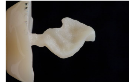
Restoration milled from an advanced lithium disilicate ceramic (CEREC T Tessera) in CEREC Primemill.
